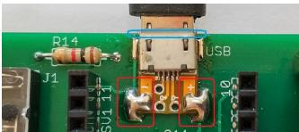
The micro-USB board is placed and aligned as shown. At the connections shown in the red rectangles, apply a lot of solder until contacts on both boards are joined. Then heat the foil on the main board below blue circled area, so that the cup becomes firmly soldered.
