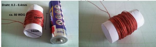
A ceramic capacitor with 1nF should also be connected in series with the coil to ground. Connect the other end to "ANT" (X2). The resonance frequency is 1.7MHz. That ranges from long wave to short wave. At higher frequencies the coil or capacitor should be adapted.
